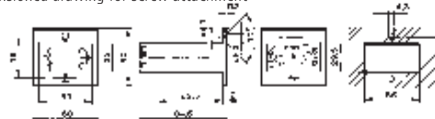
Dimensioned drawing for screw attachment
